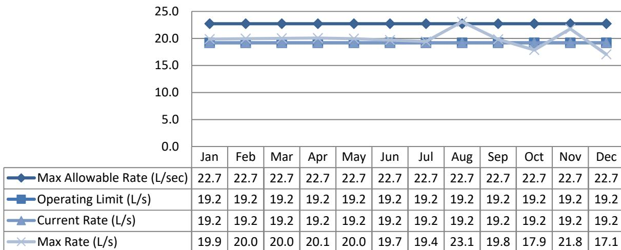
\* Brief spike in flow <1 min caused by opening the valve to fill the new above grade reservoir on August 22<sup>nd</sup>
